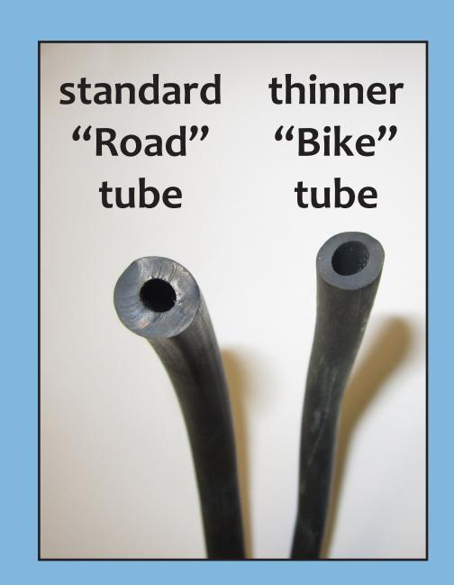
Thinner-walled "bicycle" tubes allow bicyclists to generate stronger air pulses, which have a greater likelihood of being registered as axle hits.
