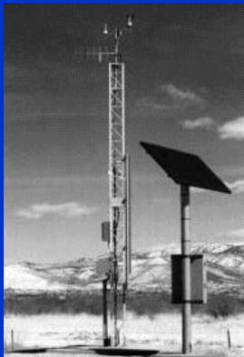
Road Weather Information Systems provide data on air and pavement temperatures, precipitation, and the amount of deicing chemicals on the pavement.
