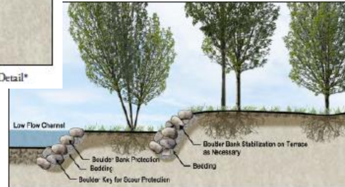
Figure 7.3 Boulder Bank Protection Detail*
