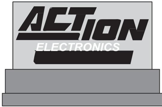
Figure 13-3: Sign area for a monument sign shall not include base, if the base is architecturally distinct.
