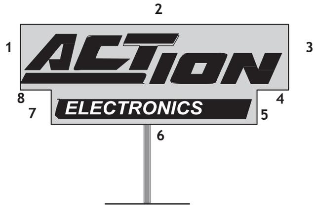
Figure 13-4: Pedestal not counted as part of sign area.
