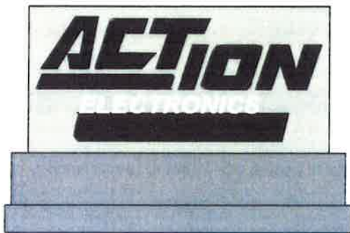
Figure 13-3: Sign area for a monument sign shall must not include base, if the base is architecturally distinct.
