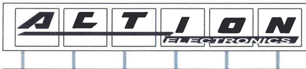
Figure 13-5: Sign area shall must include vertical and horizontal spacing between letters conveying the sign's message.
