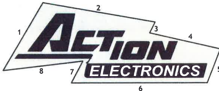
Figure 13-2: For irregularly shaped signs, area is measured as enclosed by up to 8 straight intersecting lines.
