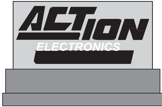
Figure 13-3: Sign area for a monument sign shall not must not include base, if the base is architecturally distinct.
