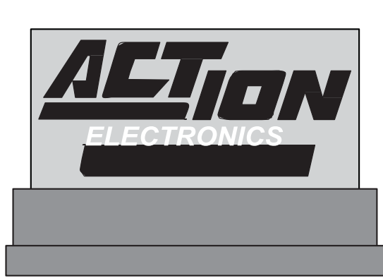
Figure 13-3: Sign area for a monument sign must not include base, if the base is architecturally distinct.
