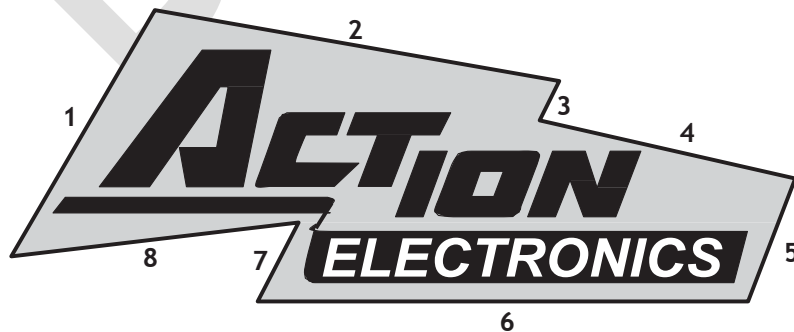
Figure 13-5: For irregularly shaped signs, area is measured as enclosed by up to 8 straight intersecting lines.
