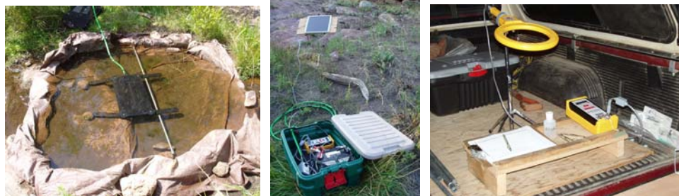
Figure 1. (left) plate antennae placed 1 cm below water surface in artificial water hole, (middle) water proof data recording station with solar panel, data reader, antennae tuner, and car battery, and (right) PIT-tagging station with ring antennae reader.
