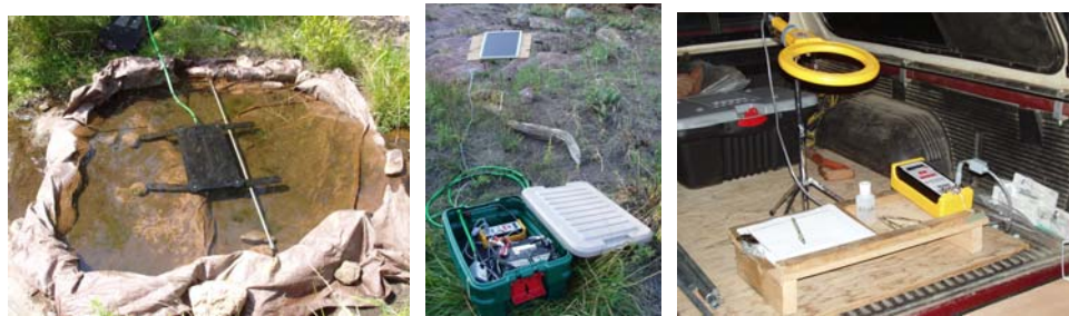
Figure 1. (left) plate antennae placed 1 cm below water surface in artificial water hole, (middle) water proof data recording station with solar panel, data reader, antennae tuner, and car battery, and (right) PIT-tagging station with ring antennae reader.
