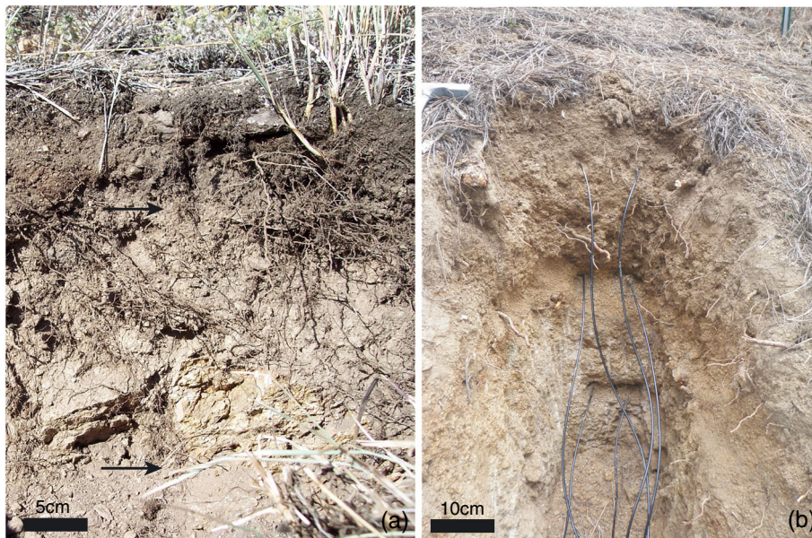
Figure 2. Photographs of representative sensor sites at Gordon Gulch and Betasso. (a) South-facing slope of Gordon Gulch prior to sensor installation. Arrows mark approximate location of sensors. Total depth of the pit is 25 cm. (b) Gully Site at Betasso with soil moisture and matric potential sensor pairs shown. Total depth of the pit is 80 cm. This figure is available in colour online at wileyonlinelibrary.com/journal/espl
