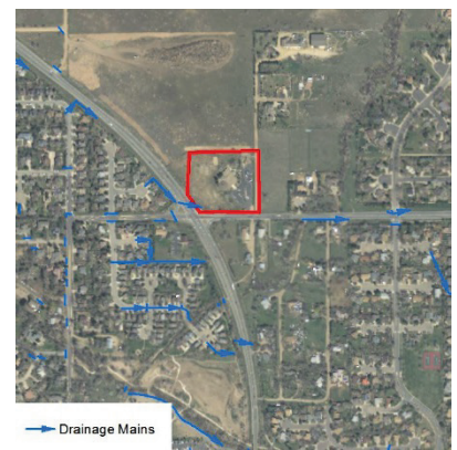
Figure 2: Existing Storm Mains
