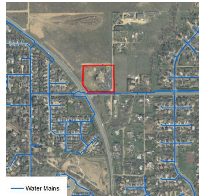
Figure 1: Existing Water Mains
