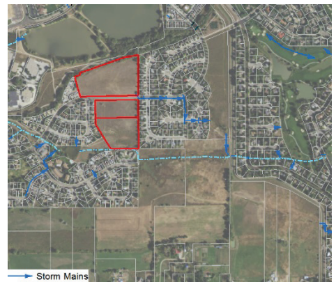
Figure 2: Existing Storm Mains
