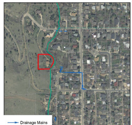
Figure 2: Existing Storm Mains
