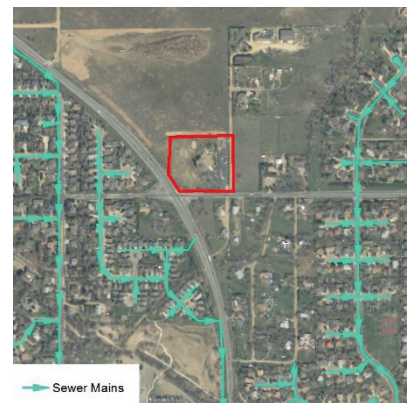
Figure 3: Existing Sewer Mains
