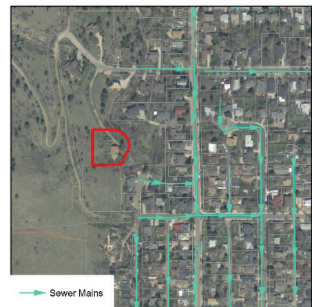
Figure 1: Existing Sewer Mains Source: Wastewater Utility Master Plan, 2009
