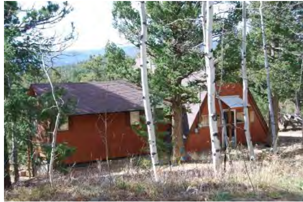
Figures 103 and 104. Two examples of A-frames with wings (modified A-frame). Left: Ronnie Lane, Unincorporated; note that the A-frame is not a double A-frame, as the roofline of the shorter wings does not extend to the ground. 203 Right: 60 Timberline Road, Unincorporated.
