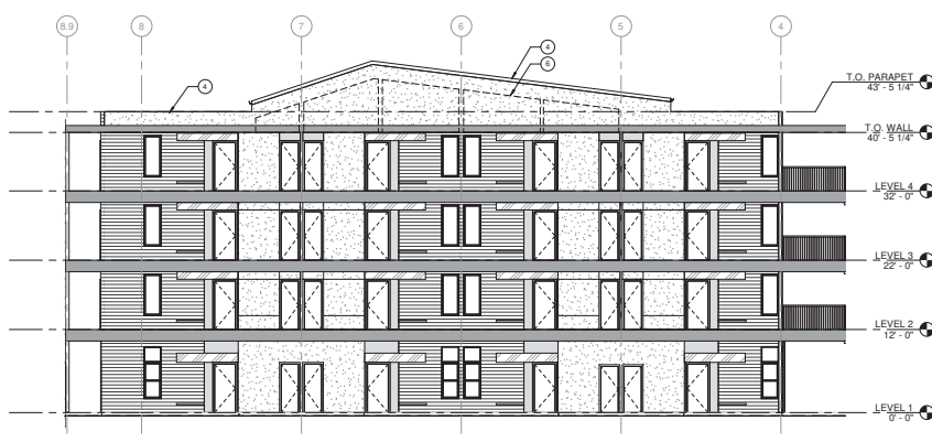
ENLARGED EAST ELEVATION OF VOLUME 3 SCALE: 1/8" = 1'-0" 4
