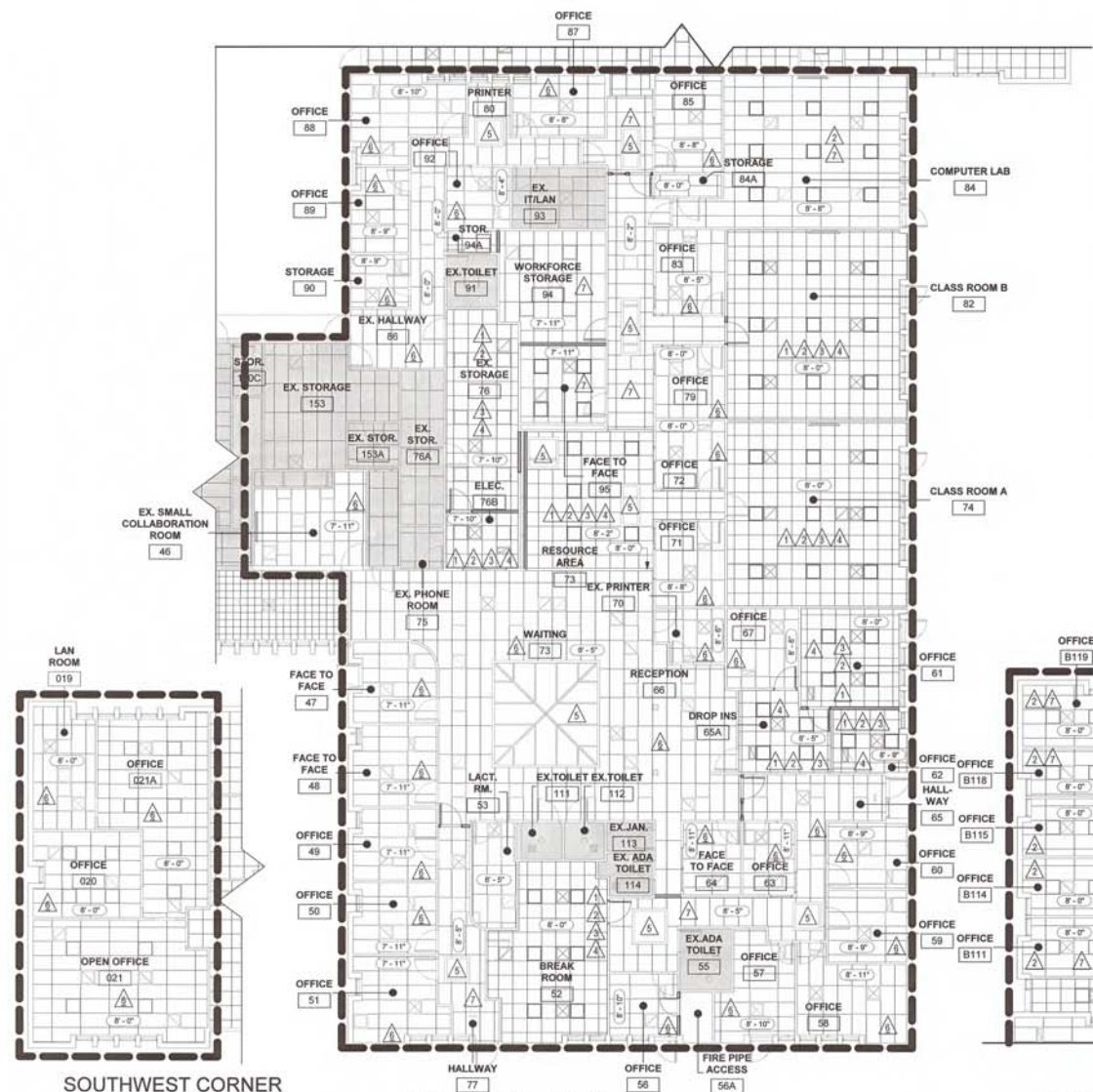
3 A102 SOUTHWEST CORNER REFLECTED CEILING PLAN 1/8" = 1'-0"
