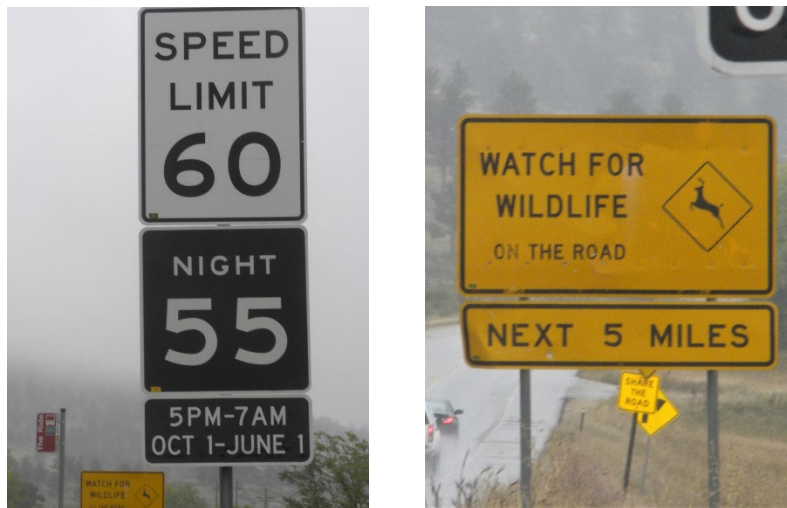
Figure 4. At left, speed limit signs highlighting the nighttime speed reduction from 2010-2012. At right, an example of one of two wildlife crossing caution signs along US 36.
