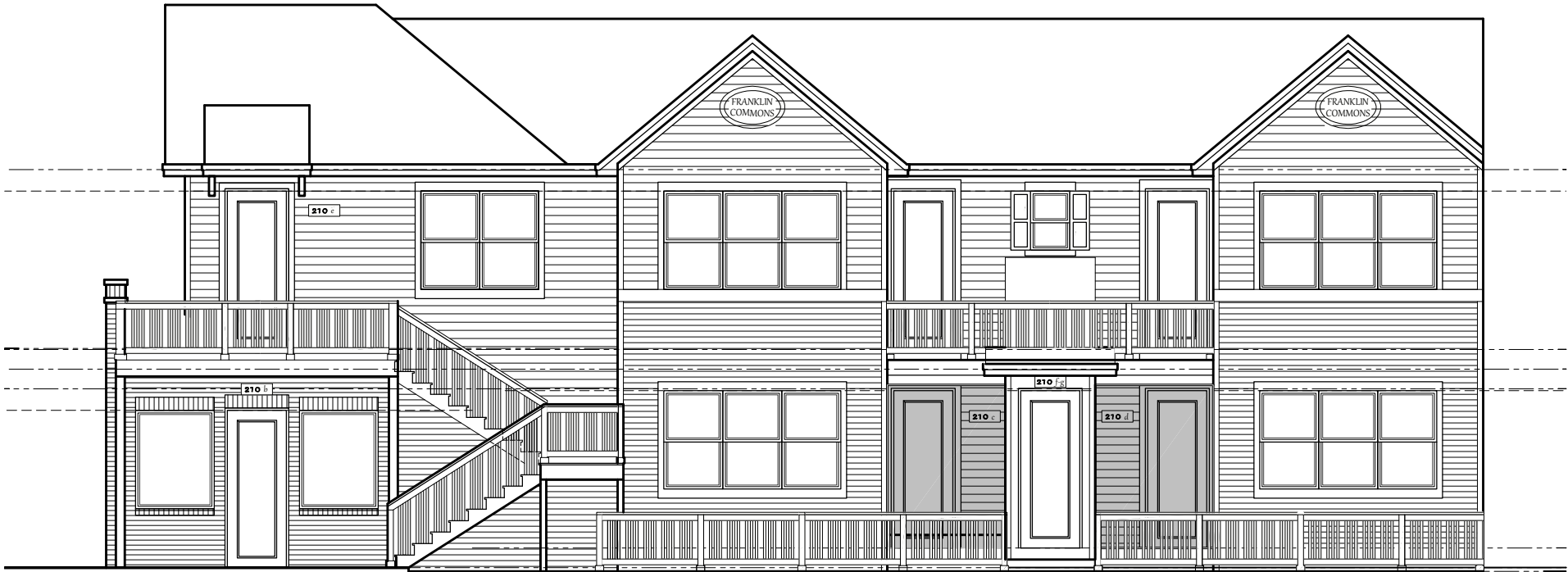
MIXED-USE BUILDING SOUTH ELEVATION (2ND AVE) SCALE: 1/4" = 1'-0"
