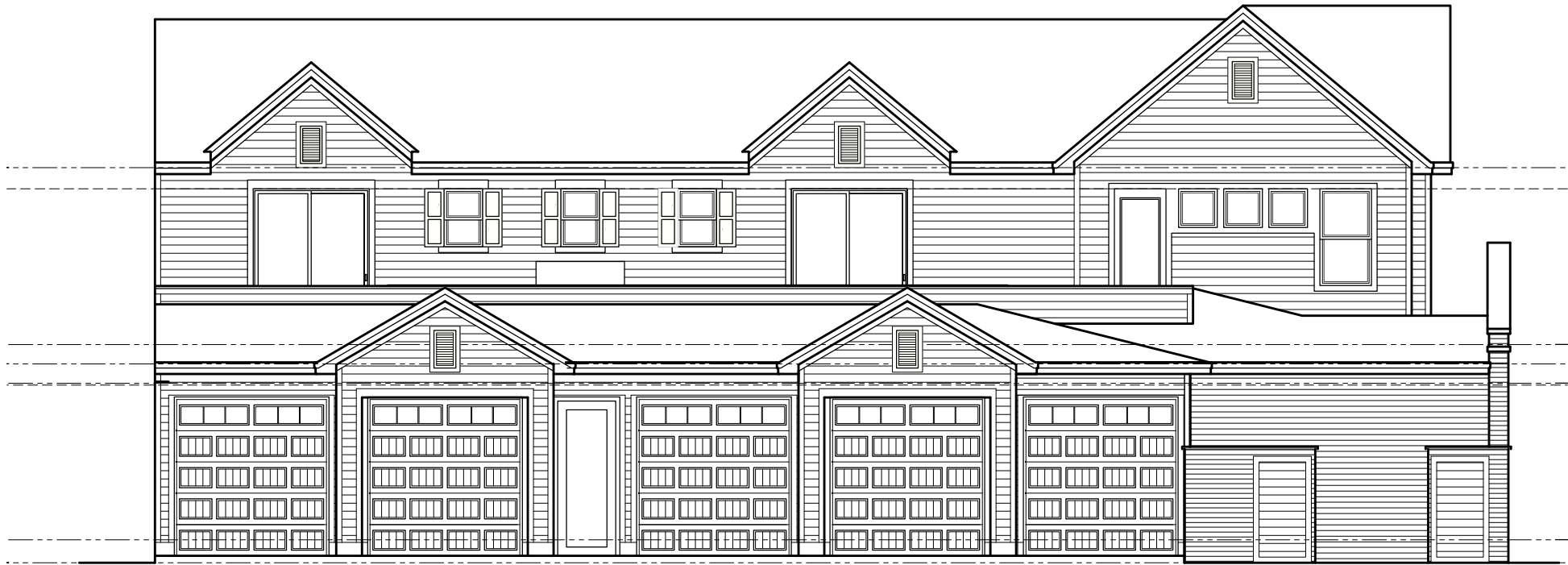
MIXED-USE BUILDING NORTH ELEVATION (ALLEY) SCALE: 1/4" = 1'-0"
