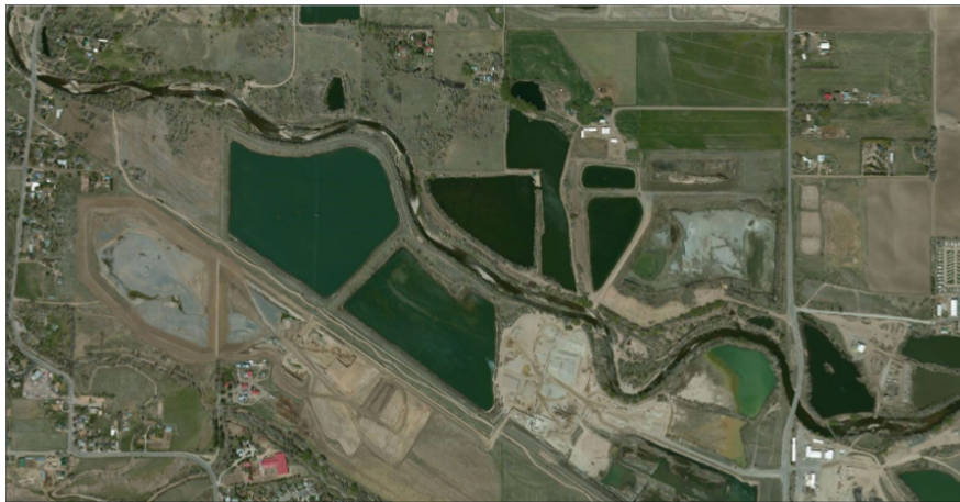
FIG. 2. Cache la Poudre River along a section of the ERM study reach, Fort Collins, Colorado, (a) in 1937 and (b) recently (circa 2005). Panel a shows a meandering channel, with a wide, unimpaired zone of channel movement across the floodplain and presence of cottonwood forests of various ages. Panel b depicts the confined channel after nearly a century of land use changes that simplified and straightened the river, reduced channel migration and the associated rejuvenation of riparian habitat, narrowed the riparian zone, and confined the channel with hardened banks and associated pit ponds following gravel extraction.
