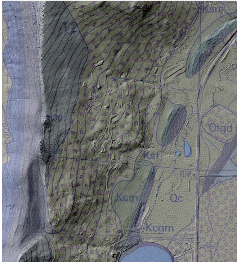
Figure 1. Lidar hillshade depicting pre-fire home sites overlain by the Geologic Map of the Lyons Quadrangle, USGS GA-1629, published in 1988. Subdivisions are within the landslide area with triangular symbols. The morphology of the landslide feature (hummocky ground) is illuminated by the Lidar image.
