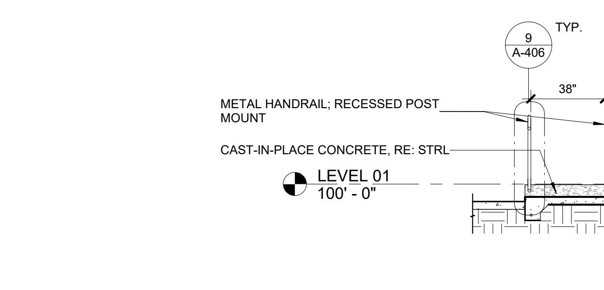
6 A-406 NORTH EXTERIOR RAMP CROSS SECTION 1/4" = 1'-0"
