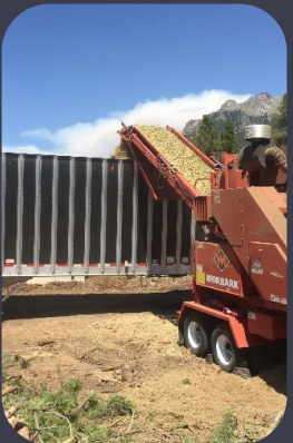
Grinding woody biomass at the Meeker Park CFSY.
