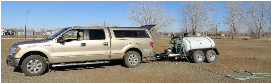
Typical 600 gallon water tank.
