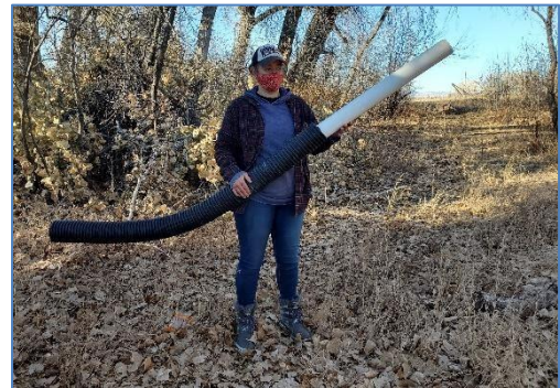
Example of a 3-inch rigid pipe inserted into a 4-inch corrugated tube.
