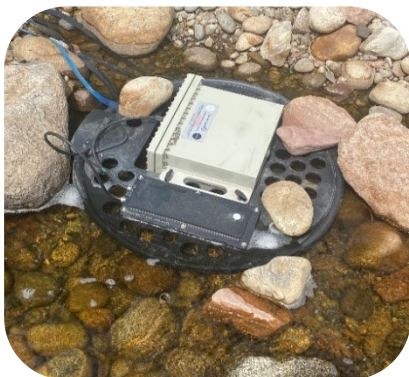
Figure 2: BioMark PIT tag reader
