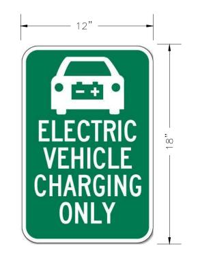
ELECTRIC VEHICLE SIGN DETAIL NO SCALE
