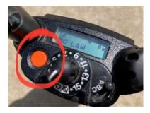
In general, the emergency button will only work if you are on an 800MHz channel such as a BC or LG (ex: BC LAW, etc). It will NOT work on an 'SO' labeled VHF channel or the Simplex 1-5 channels.
