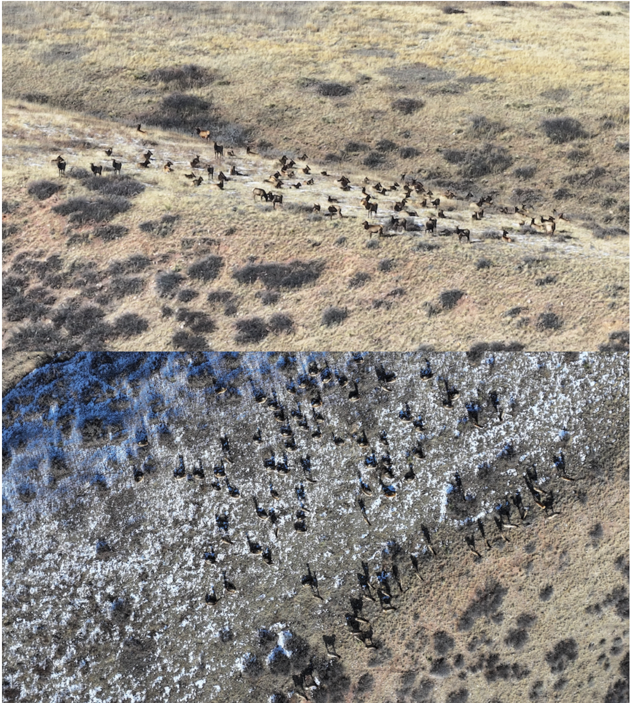
Figure 12: Comparison of oblique image to nadir image of elk herd. Above, elk were imaged from 595 m line of sight at max optical zoom (7x). The elk bedded furthest away appear bunched because of the angle and are more difficult to count. Below, the same herd imaged from 110m directly above (no zoom) reveals gaps between animals, making it easier to count individual elk once zoomed in on a computer screen.
